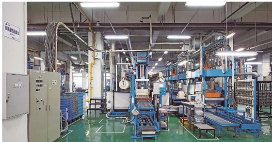
Full-automatic rotating barrel acidic zinc plating apparatus No. 6, equipped with a carrier-type after-treatment device
