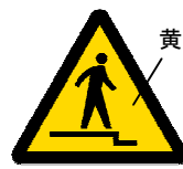
下り段差注意 Caution, uneven access/down
