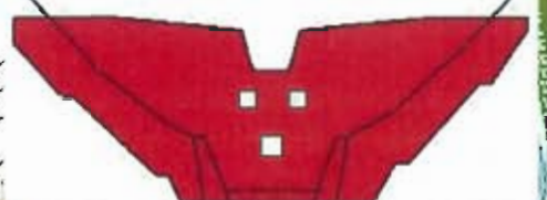
えん堤工 H=8.5m、L=40.5m
